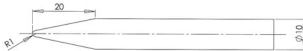
Figure A 2 Pointy probe. Shall be made of metal or other hard smooth material. Measurements in mm.
